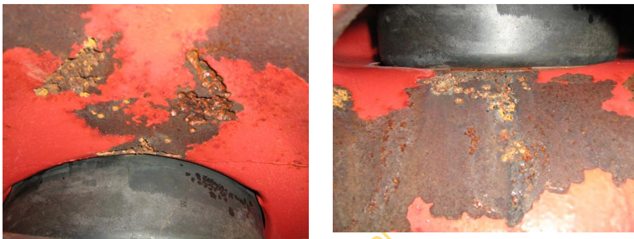
Figuur 11: Cavitieschade PSV.
